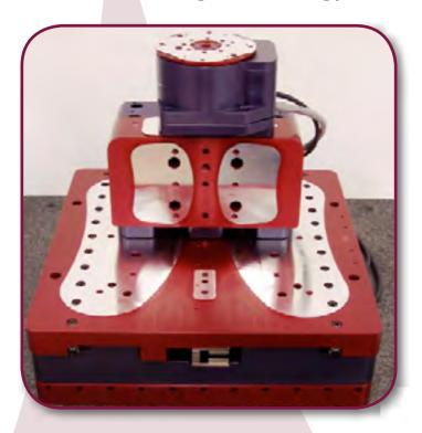
Beyond our proprietary optical design, the stage assembly is the most critical sub-assembly on the SF-100 LIGHTNING+. Stitching accuracy is critical to obtain acceptable process results and high performance of your devices. Our linear motor stage assembly offers high precision, robust design, and repeatability the will ensure very tight stiching accuracy day in and day out. Typical results from this stage include:
