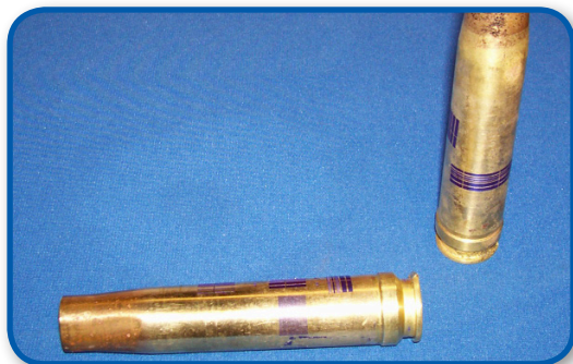
Passive Electronic Devices Patterned on Military Munitions
