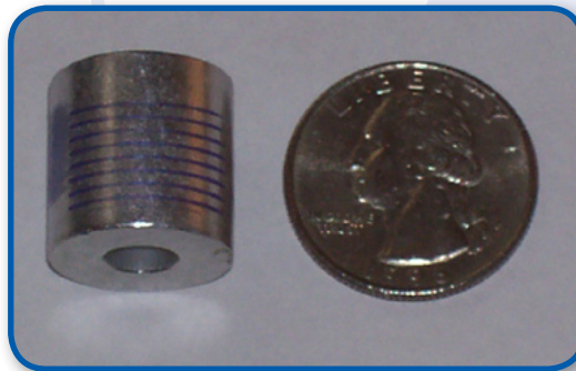
10 Micron Thick Resist Patterned on Cylinder
