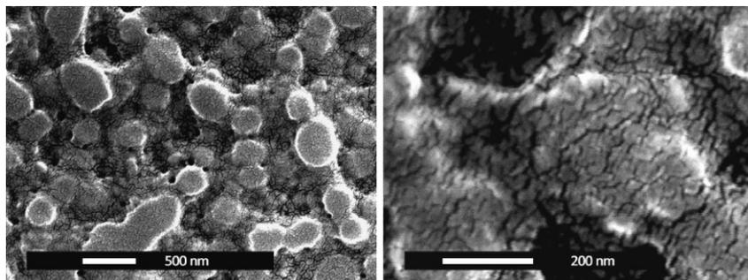
**Figure 1.** SEM images of three-dimensional porous polymer scaffold. Spin-coated polymer made with polymeric porogens is comprised of <100 nm pores and is estimated to be 1  $\mu\text{m}$  thick using confocal microscopy (data not shown).
