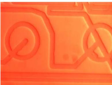
Figure 5: Microchannels etched in LCP dielectric polymer.
