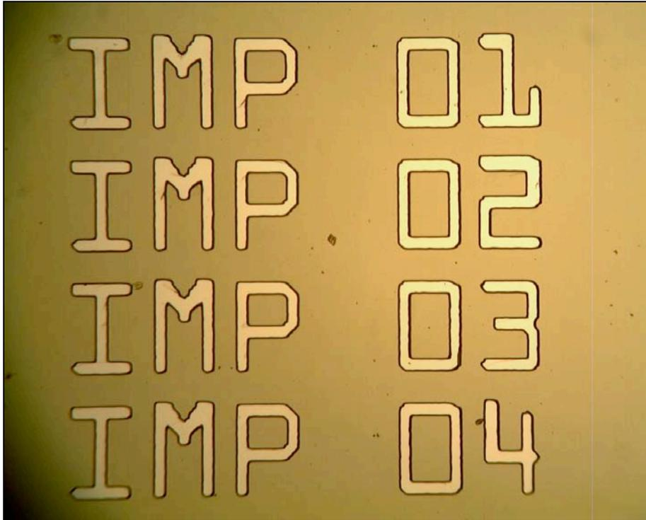
Figure 3-Individual Panel Identification Exposed on the SF-100 ELITE
