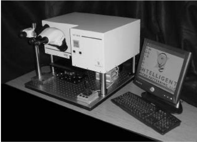
Figure 1: SF-100 Maskless Photoimaging Tool
