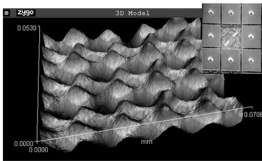
Figure 5: 3-d profile of surface roughness prior to final cure measured with Zygo interferometric system. 15  $\mu\text{m}$  peak to peak distance (red) corresponds to the individual micro-mirrors in DMD array.  $R_a = 11.2 \text{ nm}$ . (Inset) SEM image of DMD array (Texas Instruments).
