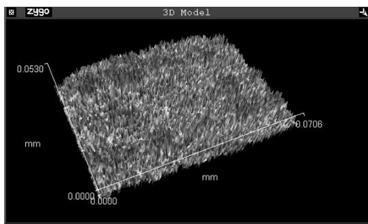
Figure 6: 3-d profile of surface roughness after final cure measured with Zygo interferometric system. Corners of mirrors are still visible, but  $R_a$  reduced to 4.4 nm.
