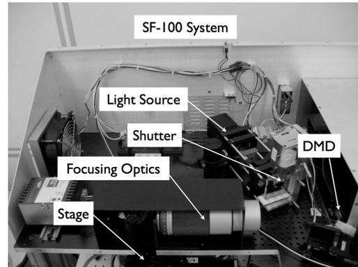
Figure 1: Layout of SF-100, DMD-based maskless lithography system used for grayscale exposures.
