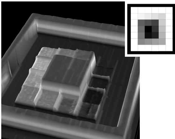
Figure 4: 3-D profile of as developed HD-8820 structure measured with Dektak Profilometer. Grayscale pattern (inset) composed of 300  $\mu\text{m}$  squares spiraling from 0% (black) in the center to 100% in 5% steps produced in Omnigraffle. Overall film thickness for this sample is 22.5  $\mu\text{m}$ .
