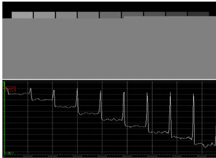
Figure 3: Example grayscale pattern generated using Omnigraffle (top). Contact profile of as developed HD-8820 film, before cure surface roughness is visible (bottom).
